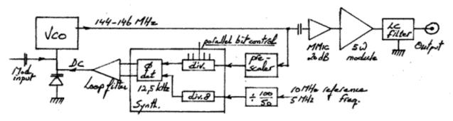
The VCO design was cribbed from a Plessey publication and uses a piece of UT-141 transmission line as an inductor. The transistor is the well-known J310 FET in common-gate configuration and the source the output. This then feeds a prescaler which in turn feeds a Motorola MC145152 synthesizer IC, (thanks Vince ZS6BTY) which offers parallel control of the internal dividers.
