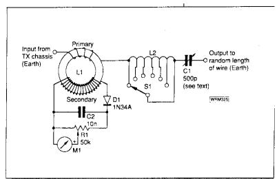
Construction tips: The tuning capacitor must be insulated from earth and chassis by the use of stand-off pillars or such like. Also the tuning shaft and knob must be insulated by a shaft extension made of a plastic potentiometer shaft. The rotary switch shaft and body is generally safe from this problem but inspect its construction to make sure.
