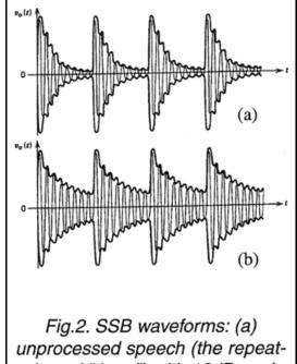
Fig.2. SSB waveforms: (a) unprocessed speech (the repeated word "three") with 16dB peakto-average ratio; (b) the same word with 6dB of compression
